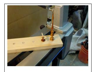
Icicles are finished off the lathe with spray lacquer. I use a strip of plywood with 3/8" hole drilled in it to hold the icicles in position to be sprayed.
