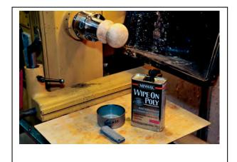
Globes may be finished on or off the lathe. On the lathe my favorite finish is Minwax Polycrylic (water based polyurethane). Several coats may be applied in one day. Smooth finish with 600 w/d after 3-4 coats. Add 3-4 additional coats. Wet sand with Micro Mesh pads to 12000 grit. Polish with McGuires 1, 2, 9, 7 grits polish (in that order!)
