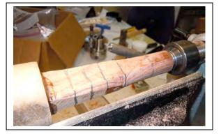
Step 1: Chuck icicle material in chuck. Bring up tailstock for initial shaping. Initially remove corners of stock and rounding out only at tailstock end.
