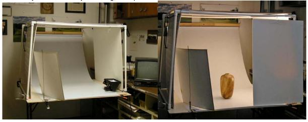
Photo 1. Frame is ½" PVC pipe, sides measure 34"x34" and top is 44" wide. Backdrop is white vinyl roll-up window shade. I often plug camera video into this monitor for enhanced view of camera image.
